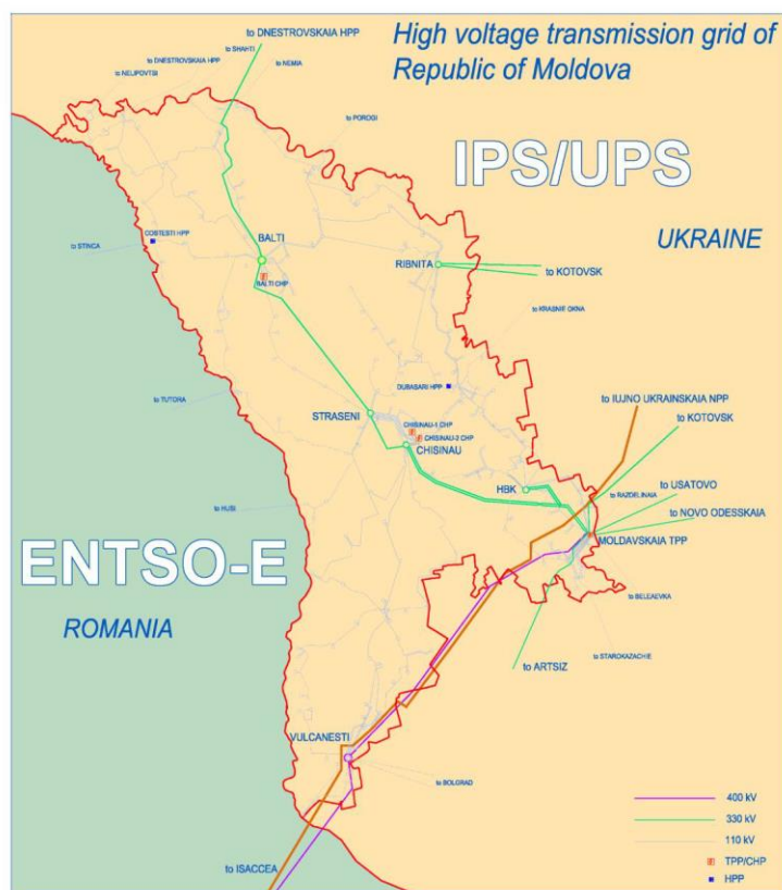
Figure 4: Moldovan electricity grid
